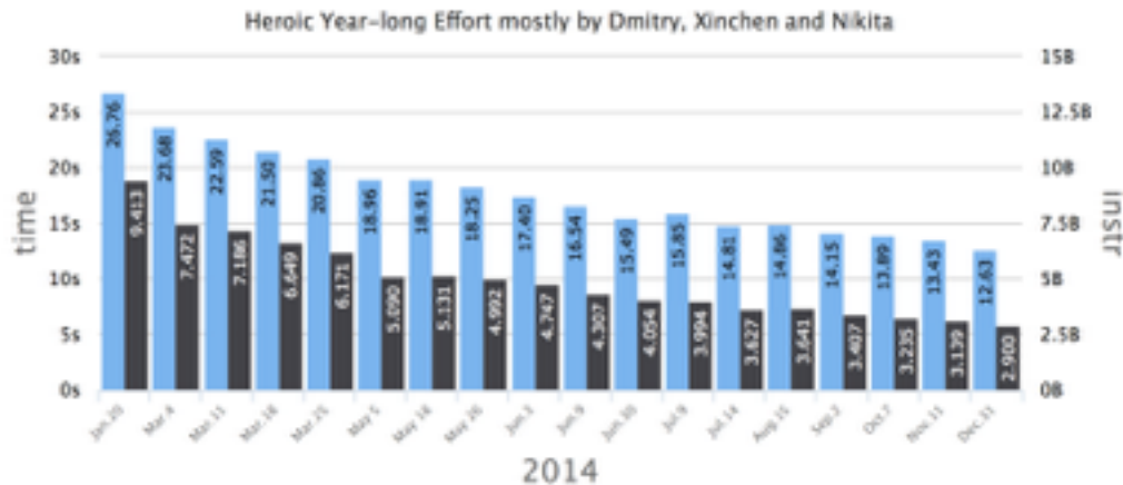
Time and number of machine instructions for 100 requests against Wordpress-3.6.0 front page
